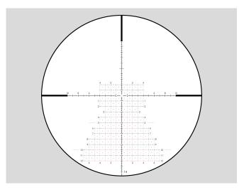
The GR<sup>2</sup>ID reticle has been designed in collaboration with international Precision Rifle Competitors, where focus has been on providing as much information to the competitor as possible, while reducing perceived clutter to a minimum. The GR<sup>2</sup>ID reticle features 4 distinct areas of design; the Base Reticle, the Ballistic Grid, the Hold Over/Under Grid and the Illumination Tree.
