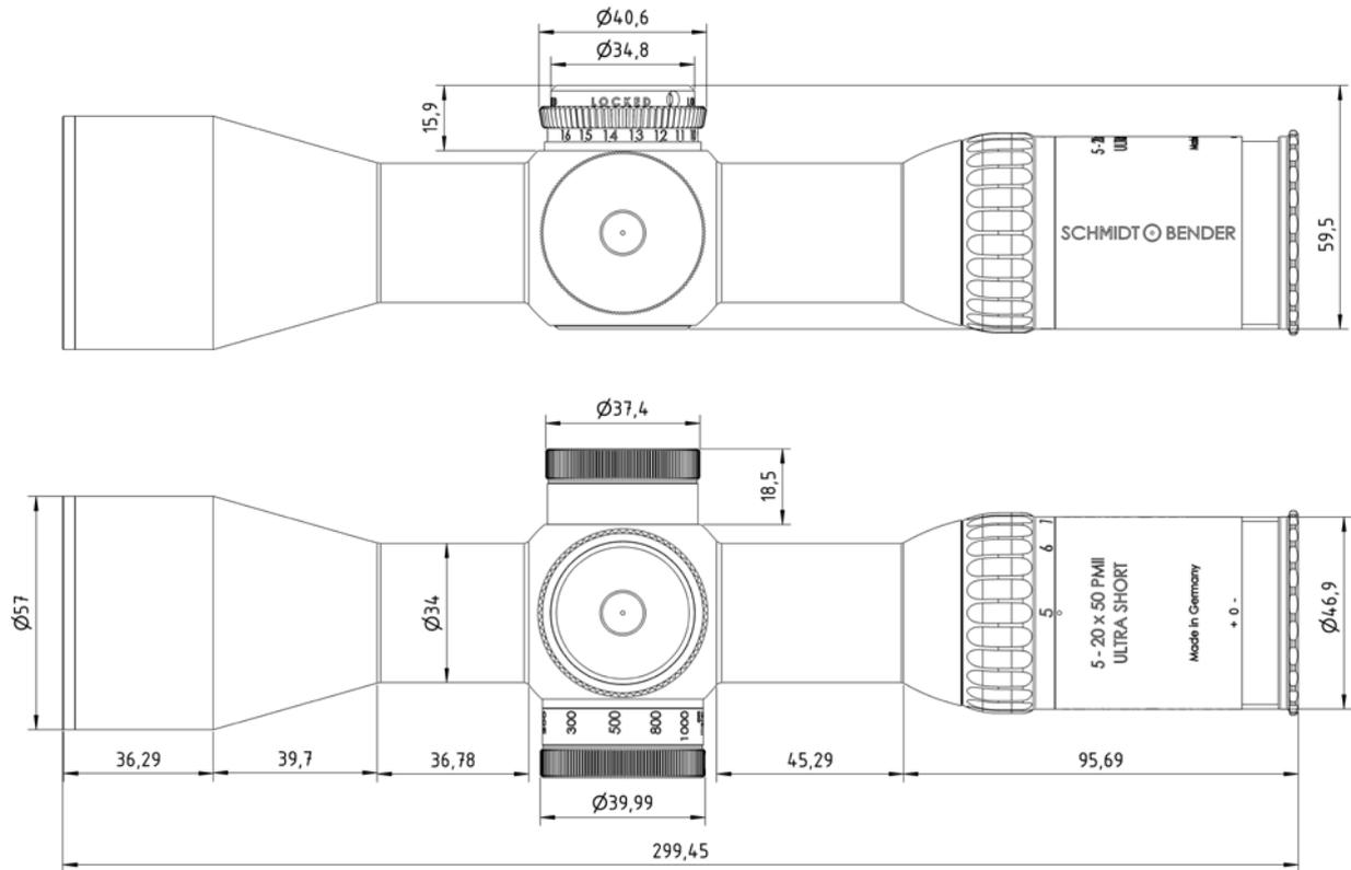
Abmessungen in mm
